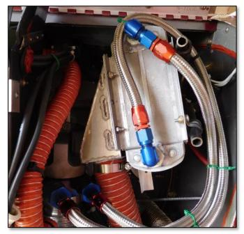
With all the necessary parts and hoses at hand the new oil cooler was installed in the space between the fire wall and the engine baffle on the port side of the engine bay. (That's the left side for you land lubbers.) On the Monday morning after the Christmas Party, Phil tested the new oil cooler system during a 1.8 hour flight. He was very happy to report that the oil temperature did not go above 190 degrees during the entire flight.
